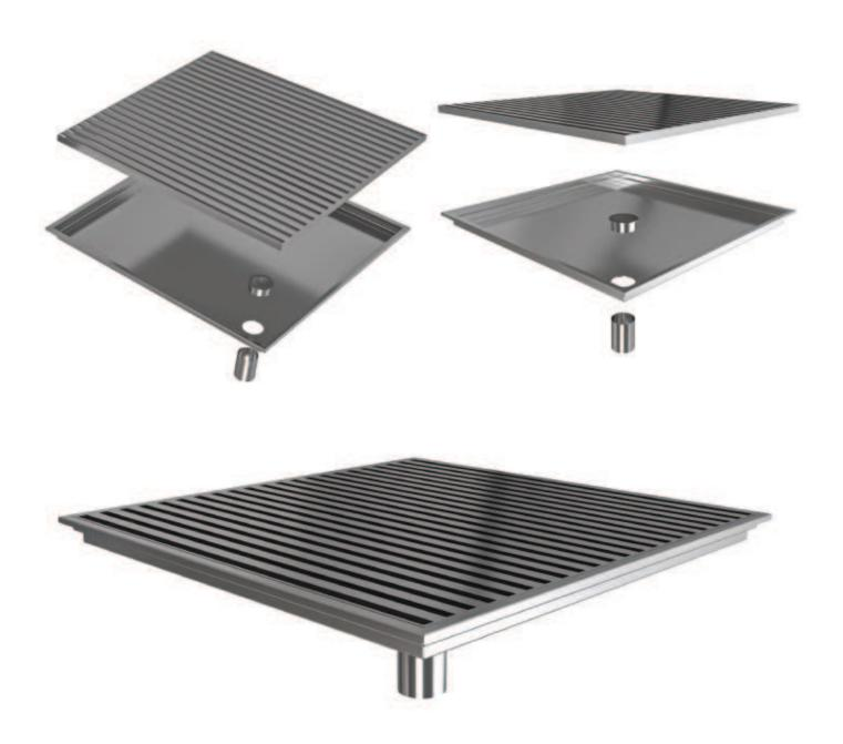
It is made of AISI 304 - 316 quality stainless steel sheet. It is hygienic, does not hold grease and dirt, and is easy to clean. There is a special siphon system that prevents odor, mice and insects from the installation. There is an anchor system so that it can be fixed perfectly to the ground during installation. Grill outlet diameters are 50 - 70 - 100 cm PVC.
