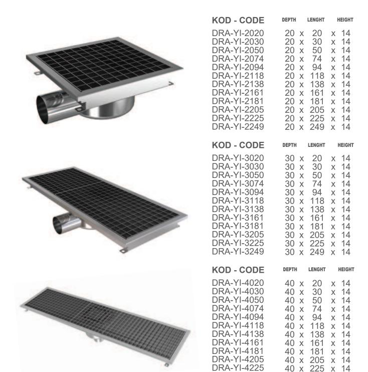
It is made of AISI 304 - 316 quality stainless steel sheet. It is hygienic, does not hold grease and dirt, and is easy to clean. There is a special siphon system that prevents odor, mice and insects from the installation. There is an anchor system so that it can be fixed perfectly to the ground during installation. Grill outlet diameters are 50 - 70 - 100 cm PVC.
